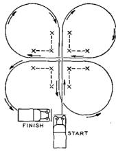
(The figure should be symmetrical, with the stakes placed to allow a side clearance of approximately 18 inches on the turn. Actual placement of the stakes should be determined from the performance of a pilot vehicle, since the total space required for the turn depends upon the type of vehicle used.)
